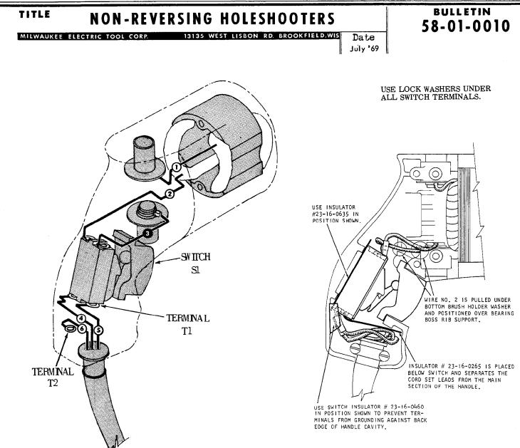
NOTE: ALL LEADS MUST BE HELD TO ± 1/8" ALL FIELD LEADS TO BE MEASURED FROM AND PERPENDICULAR TO LAMINATIONS. ALL LEAD LENGTHS ARE BEFORE STRIPPING.
